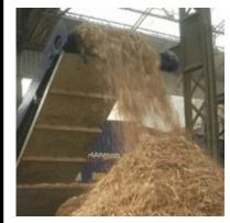
Chipboard is manufactured by mixing wood particles or flakes together with a resin and forming the mixture into a large sheet.
