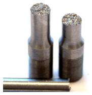
Cast Iron is a less ductile metal and is brittle due to its higher carbon content.
