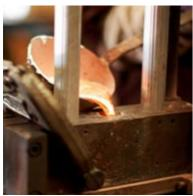
Cast iron is iron or a ferrous alloy which has been heated until it liquefies, and is then poured into a mould to solidify.
