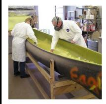
Laying up is the term used for the process involved in manufacturing with GRP.
