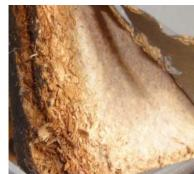
Chipboard is very prone to expansion and discoloration due to moisture.
