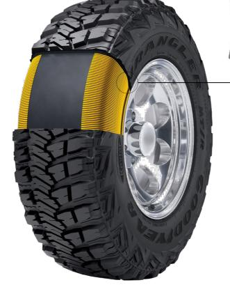
Kevlar fibres offer superb puncture, abrasion and tear resistance. Other benefits include a quieter ride and a reduction in rotational weight, which can help decrease engine strain, and typically results in improved fuel efficiency.
