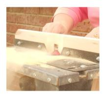
When cut MDF produces a lot of dust which is the subject of some safety concerns. A dust mask should be worn.
