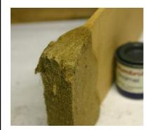
MDF can be easily damaged by moisture.
