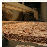
Sterling board is formed by taking shredded or flaked timber particles, adding water-resistant resins and then compressing them into layers.
