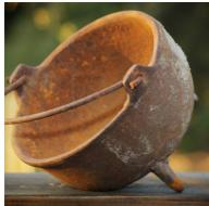
Cast Iron can have poor corrosion resistance.
