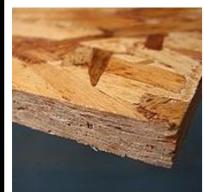
Sterling board is a material with high mechanical properties that make it particularly suitable for load-bearing applications in construction.
